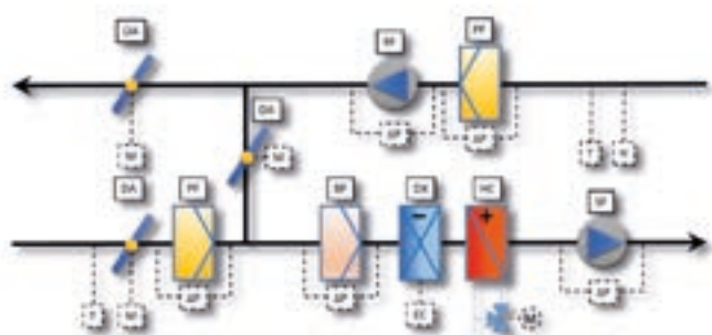
Mixing Air Handling Unit Control Flow Chart
