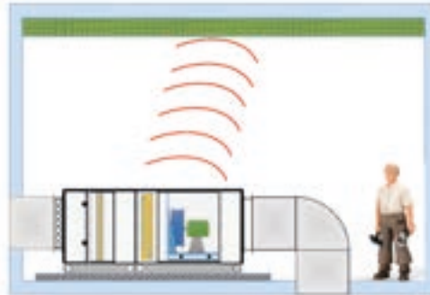
Absorption: sound energy propagating in the air is converted to heat energy.
